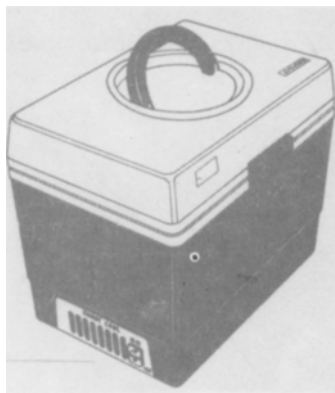
Fig. 1 Sketch of the Sunny Cool box which was used as a PMC calorimeter
